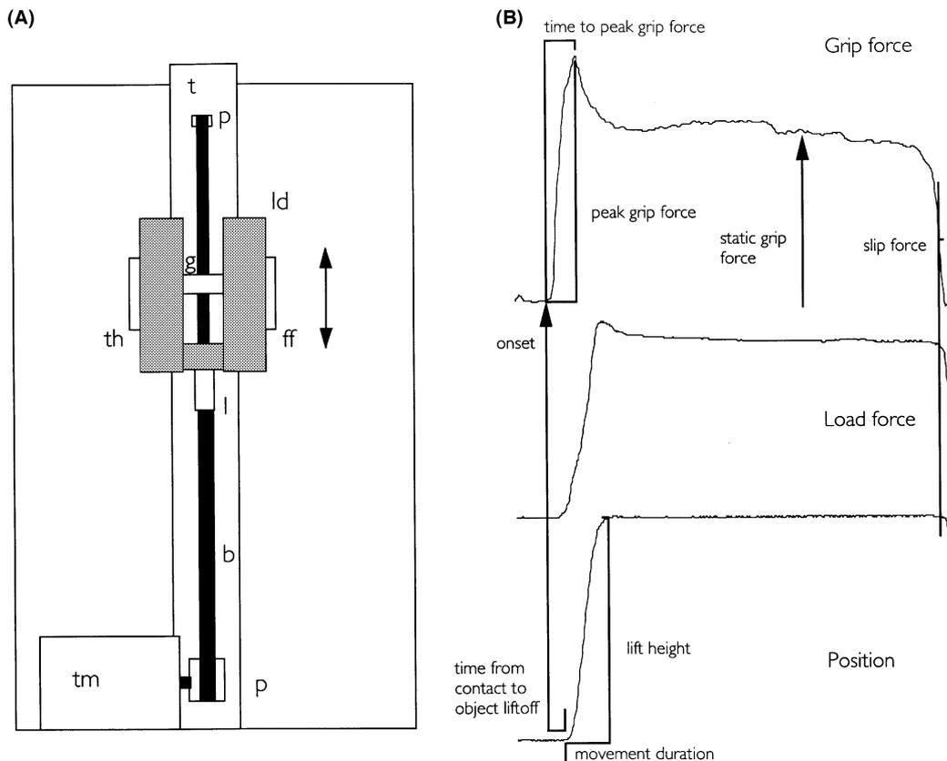
**Fig. 1** (A) The lifting apparatus.  $\beta$  = connecting band; ff = forefinger grip; g = grip force transducer; l = load force transducer; ld = load; t = track; th = thumb grip; p = pulley; tm = torque motor. (B) Grip force, load force and position traces from a typical normal lift, illustrating the parameters measured for each lift.
